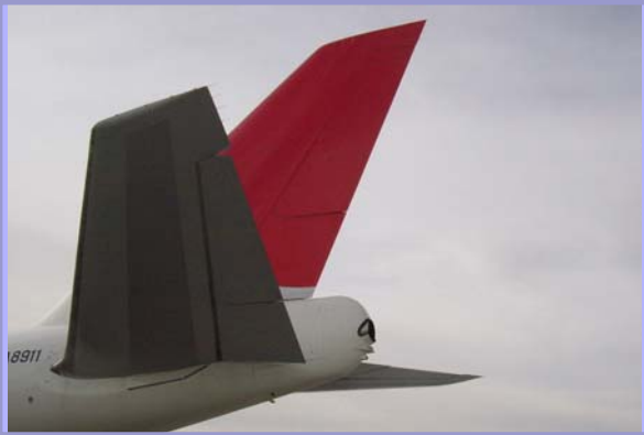
APU (Auxiliary Power Unit)
